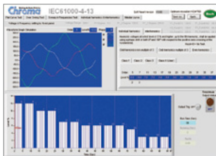
Voltage Harmonic & Interharmonic Test
